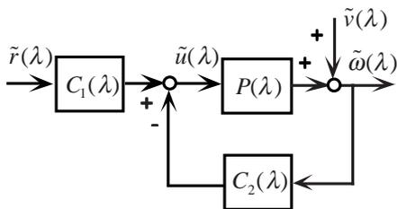
Fig. 1. Configuration of constant-speed-rotation control system.
