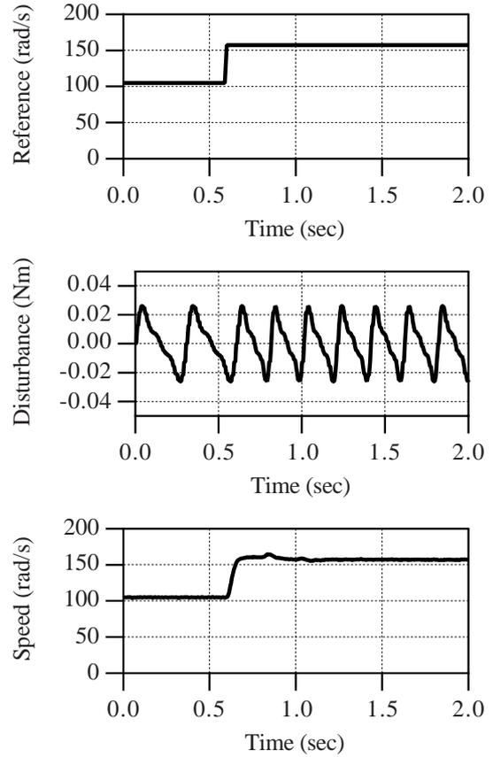
Fig. 6 Response to change of the speed setting.
