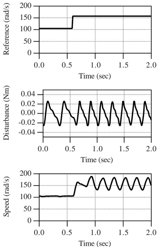
Fig. 7 Response of constant-speed-rotation control system designed in the time domain.
