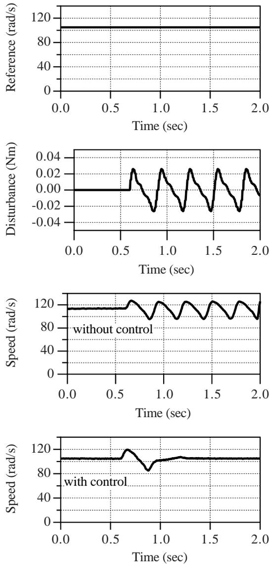
Fig. 5 Response to disturbance for a standard speed setting.
