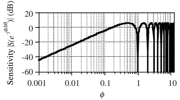
Fig. 4. Sensitivity characteristics of the designed constant-speed-rotation control system.
