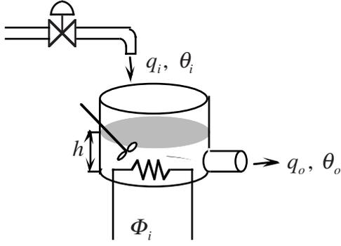
FIGURE 1: The tank system.
