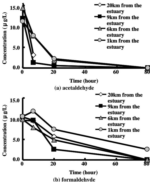
Fig. 9 Concentrations of Aldehydes on Biodegradation Experiment in river water with different salinity
