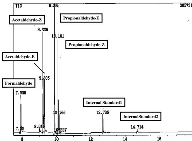
Fig. 3 Chromatogram of GC/MS measurement
