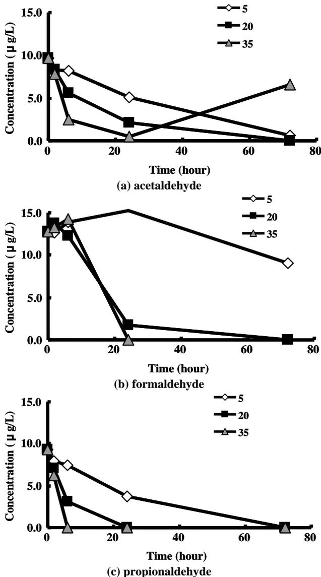
Fig. 7 Concentrations of Aldehydes on Biodegradation Experiment at Different Temperature
