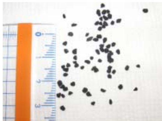
Fig. 2 Granular activated carbon
